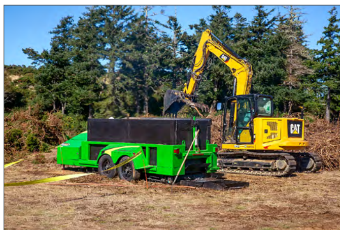
Figure 2.1. This biochar production unit 1 and loader are an example of moderate-scale biochar production. Here, biomass resulting from removal of invasive gorse is converted to biochar in Bandon, Oregon. Conversion to biochar inhibits the spread of the invasive plant. (Photo: U.S. Forest Service Region 6 State & Private Forestry)
