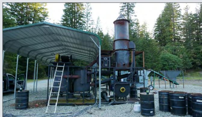
Figure ES-9. This relocatable gasification system was set up for Redwood Forest Foundation, Inc. in Andersonia, California in 2017 and is an example of a moderate-scale system. (Photo: Arne Jacobson)
