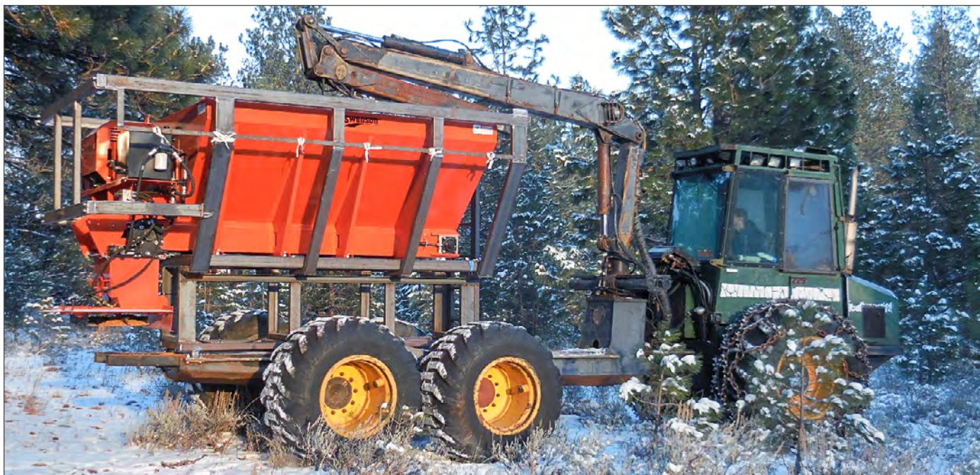
Figure 2.2. The USDA Forest Service National Technology Development Center developed a biochar spreader that can be used to apply biochar to log landings or skid trails, seen here working on the Lubrecht Experimental Forest in Montana. This equipment can work on slopes up to 35%. (Photo: USDA Forest Service)
